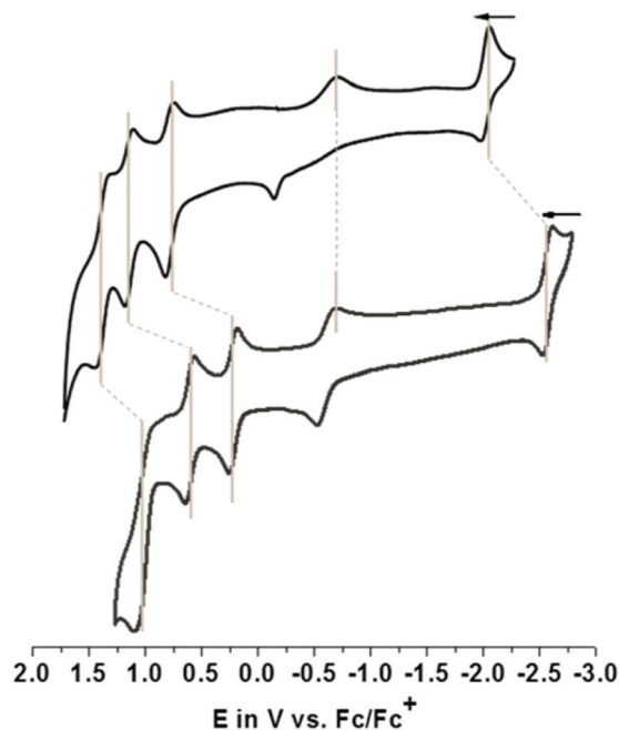
Fig. 6 Cyclic Voltammograms of 1 (top), and 4 (bottom) in acetonitrile. Conditions: 0.1 M TBAPF 6 as supporting electrolyte; Glassy carbon (working), Pt wire (counter) and Ag/AgCl (reference); Scan rate: 100 mV s -1 .
